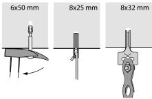
When the eye in the Ceiling Anchor is exposed to tension, it will expand in the material
