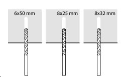
1] Drill a hole in correct diameter and depth
